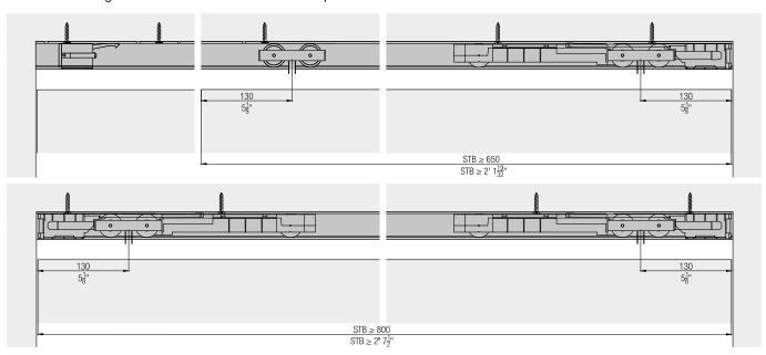
Fitting for top-running wooden doors up to 100 kg (220 lbs.), with surface mounted running track. Optionally with soft and self closing mechanism. Ceiling mounting. Wall pocket solution.
