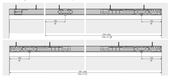
Fitting for top-running wooden doors up to 100 kg (220 lbs.), with surface mounted running track or running track flush with the ceiling. Optionally with soft and self closing mechanism. Ceiling mounting. Wall pocket solution.
