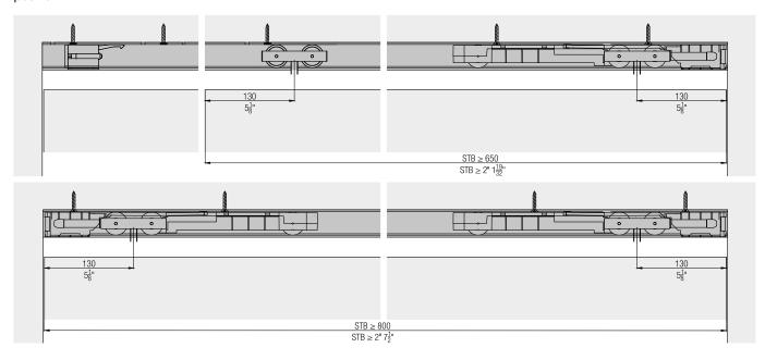
Fitting for top-running wooden doors up to 100 kg (220 lbs.), with surface mounted running track or running track flush with the ceiling. Optionally with soft and self closing mechanism. Wall or ceiling mounting.
